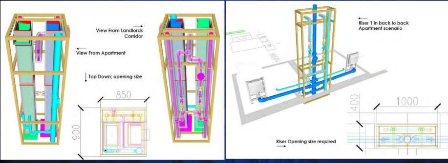
Typical Riser Used in the construction of this housing project in the UK. As seen, risers were used throughout the building for ventilation, water and electrical purposes. In the process of industrialisation, the main objective is to standardise our product in order to reduce the design cost, optimise production cost and introduce self delivery/off site solutions.
