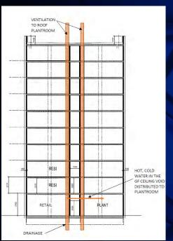
•AHU with Thermal Wheel is located on the roof for each core.
