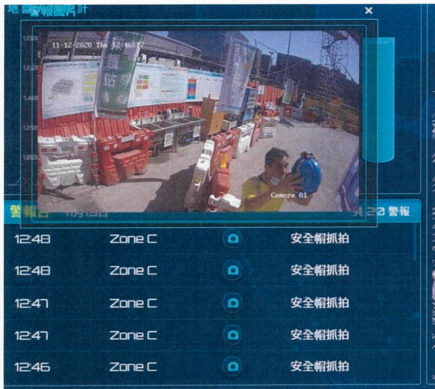
CCTV+AI safety monitoring system
