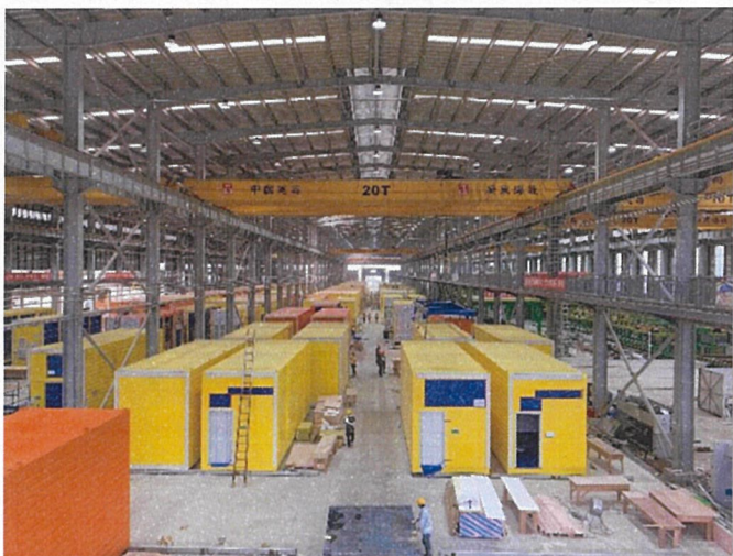
MiC Unit Manufacturing Factory
