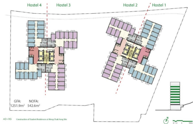
Figure 3-16 Modularisation of the floor layout of a reference student hostel
