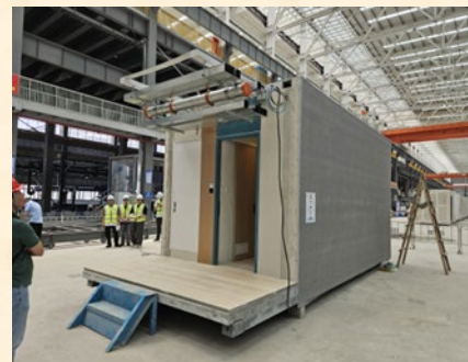
Volumetric pre-finished modules
