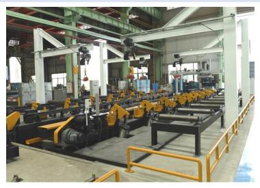
装配柔性夹具 Assembling the flexible fixture
