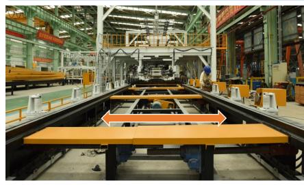
产线宽度自动调节 Automatic adjustment of production line width
